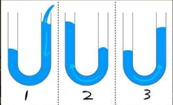
The diagrams show a U-tube with blue liquid. In diagram 1, the liquid is higher on the right side. In diagram 2, the liquid is higher on the left side. In diagram 3, the liquid is higher on the right side again, illustrating a continuous oscillation.
