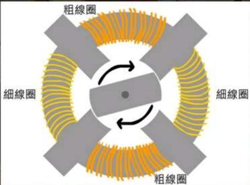
The diagram shows a central rotor with two curved poles. It is surrounded by four stator poles. The top and bottom poles are labeled '粗線圈' (thick coils) and the left and right poles are labeled '細線圈' (thin coils). Arrows indicate the rotation of the rotor.
